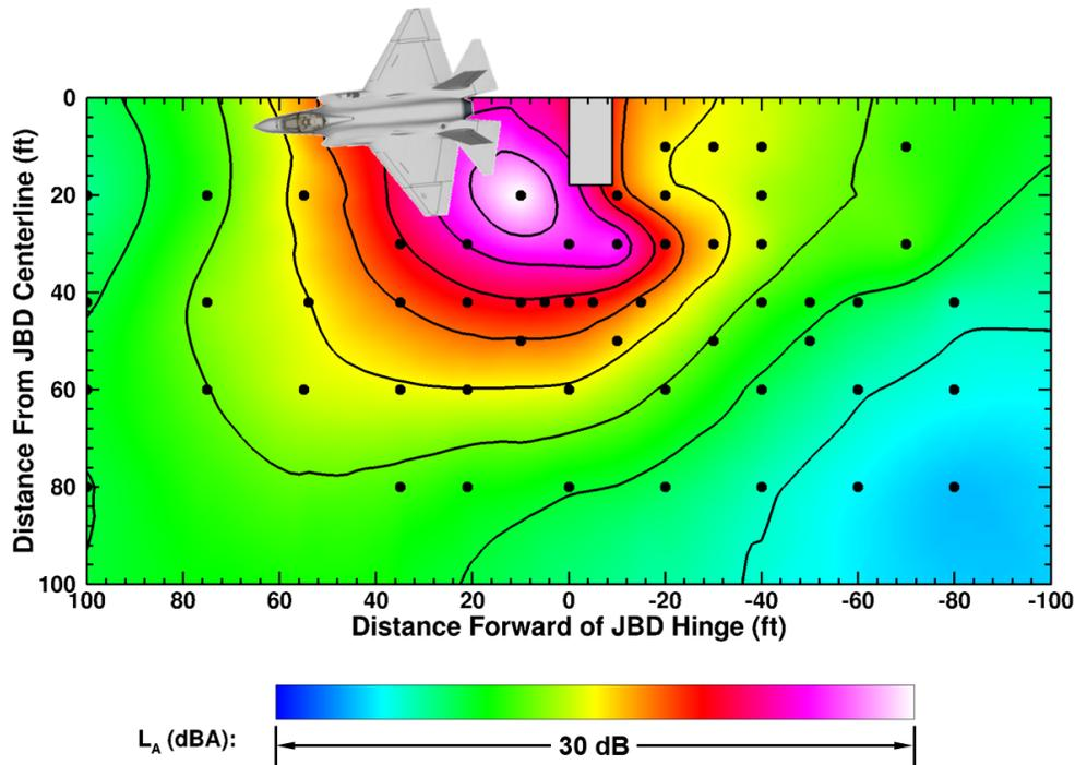
Figure 10. Afterburner power  $L_A$  contours in the near field of Catapult 1. Black circles denote microphone locations.
