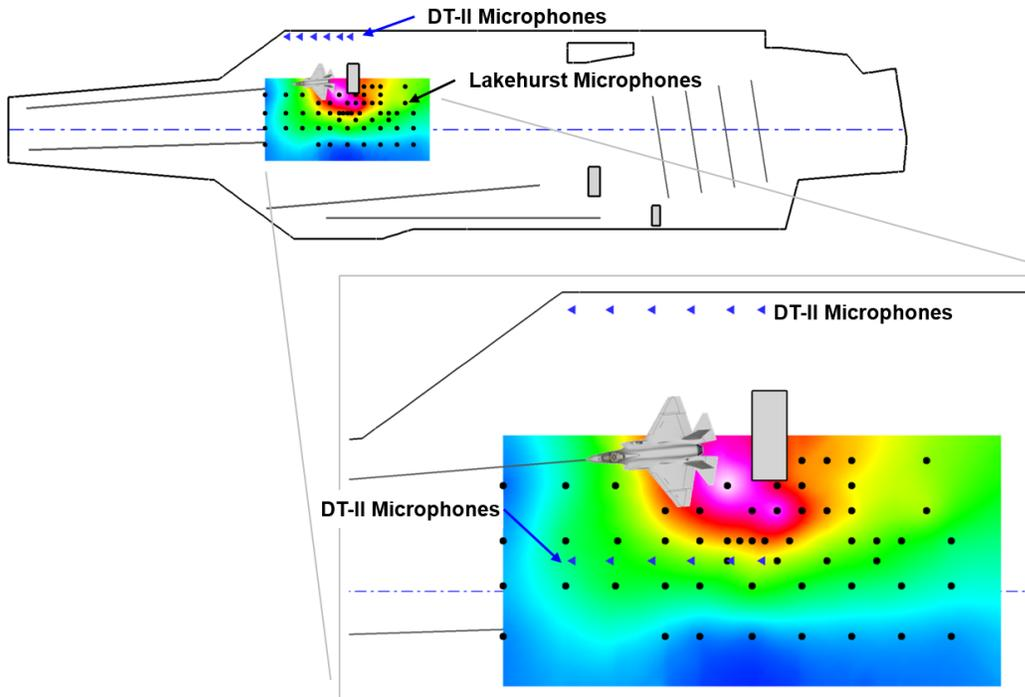
Figure 11. Land-based Catapult 1 Afterburner power  $L_A$  contours overlaid on a sketch of an aircraft carrier flight deck. Black circles denote land-based microphone locations. Blue triangles denote carrier-based microphones.
