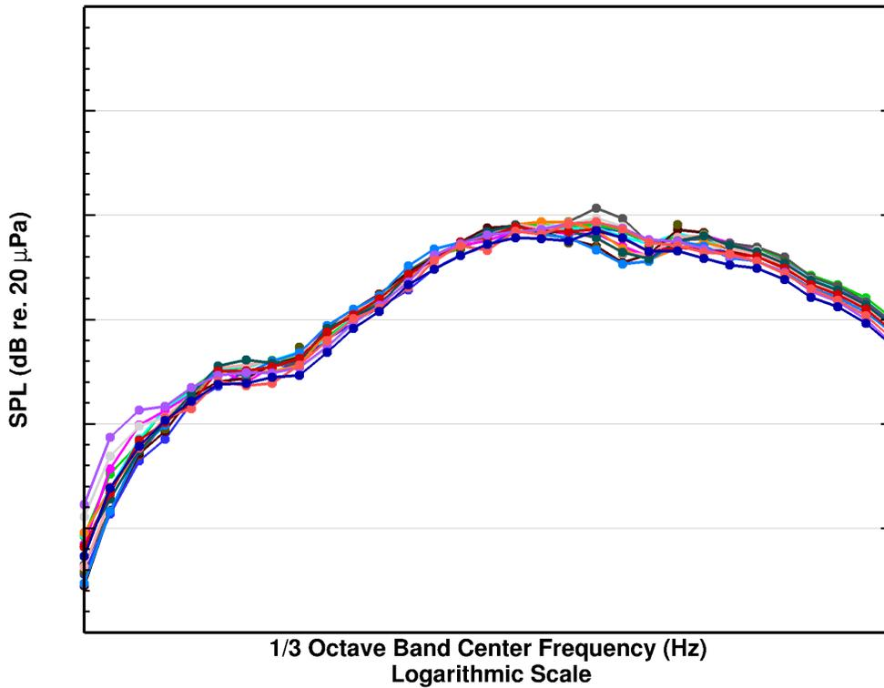
Figure 13. Carrier-based Catapult 2 military power one-third octave band spectra for the microphone located at  $(x, y) = (19.1, 125.0)$ . Distances are measured in feet, and are referenced to the center of the JBD hinge line.
