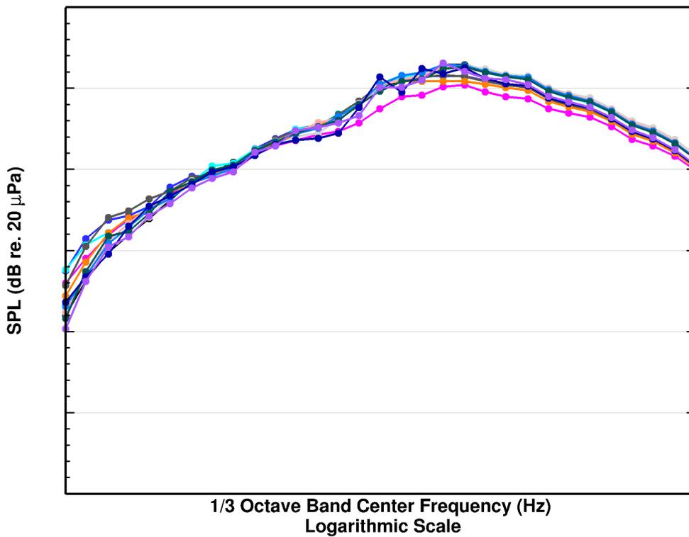
Figure 14. Carrier-based Catapult 1 afterburner power one-third octave band spectra for the microphone located at  $(x, y) = (8.33, 50.0)$ . Distances are measured in feet, and are referenced to the center of the JBD hinge line.
