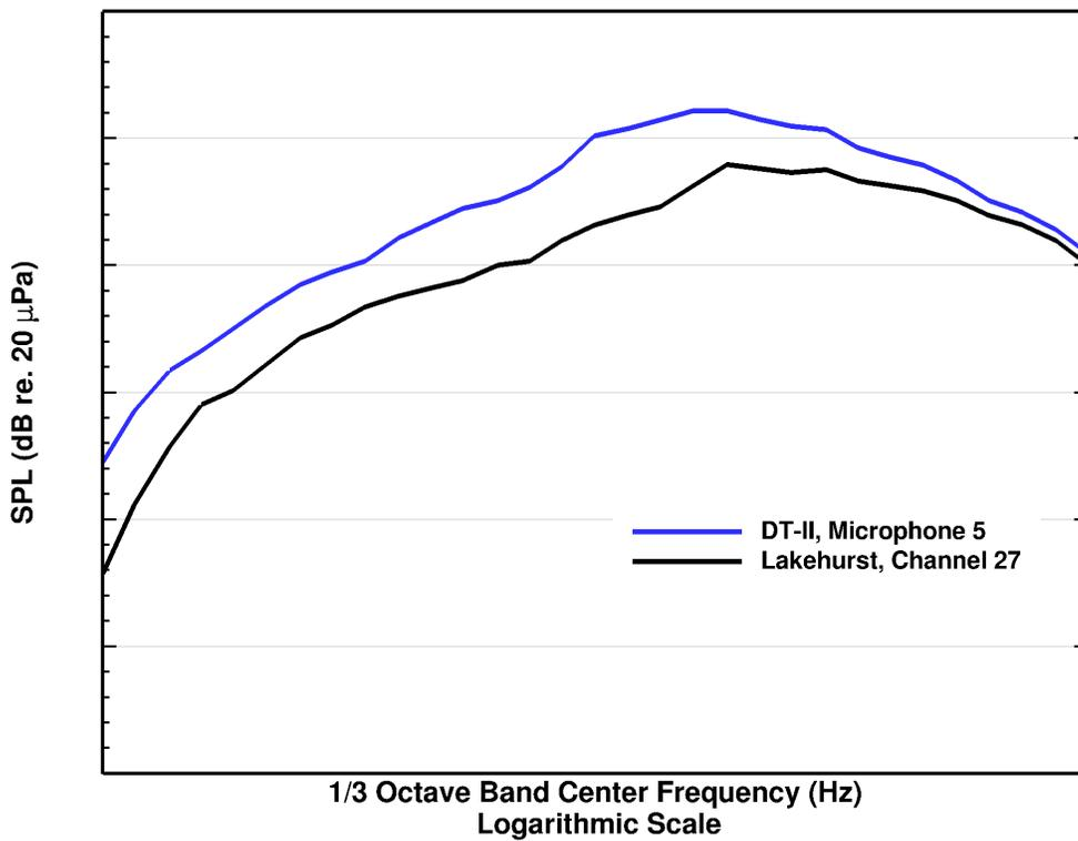
Figure 16. Comparison of land-based and carrier-based Catapult 1 afterburner power one-third octave band spectra for the land-based microphone located at  $(x, y) = (10.0', 50.0')$ , and the carrier-based microphone at  $(x, y) = (8.3', 50.0')$ .
