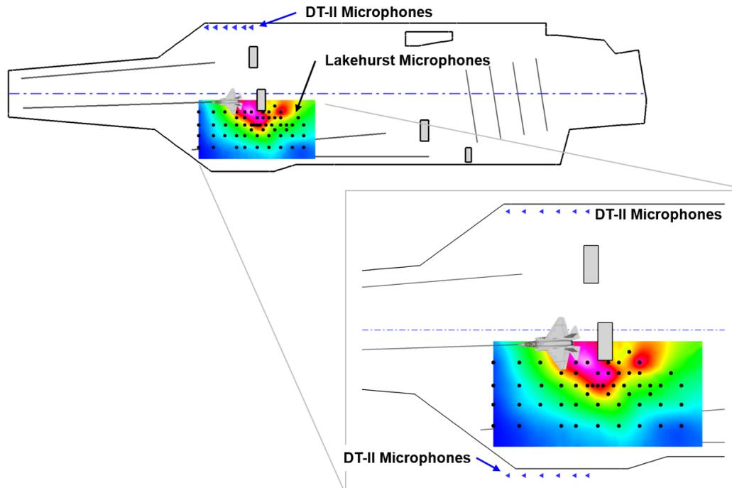
**Figure 8.** Catapult 2 Military power OASPL contours overlaid on a sketch of an aircraft carrier flight deck. Black circles denote land-based microphone locations. Blue triangles denote carrier-based microphones.
