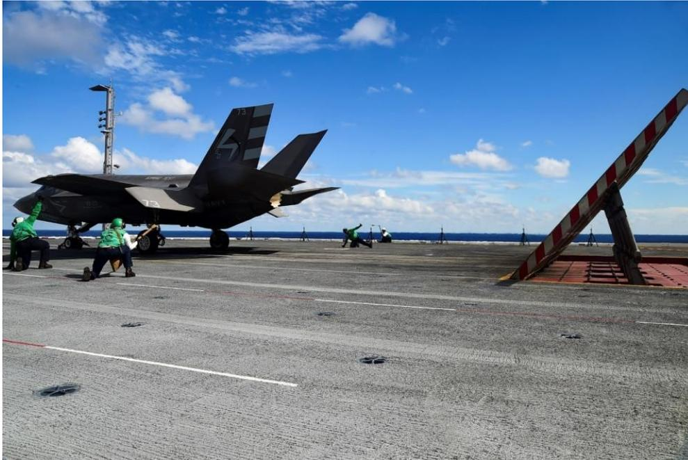
**Figure 6.** Portable (foreground, aft of wingtip), and fixed (background, on tripods) microphone systems employed on DT-II.
