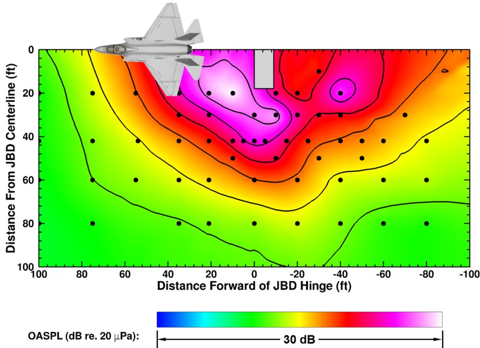
Figure 7. Military power OASPL contours in the near field of Catapult 2. Black circles denote microphone locations.
