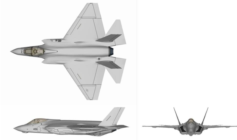
Figure 1. F-35C Configuration Three-View
