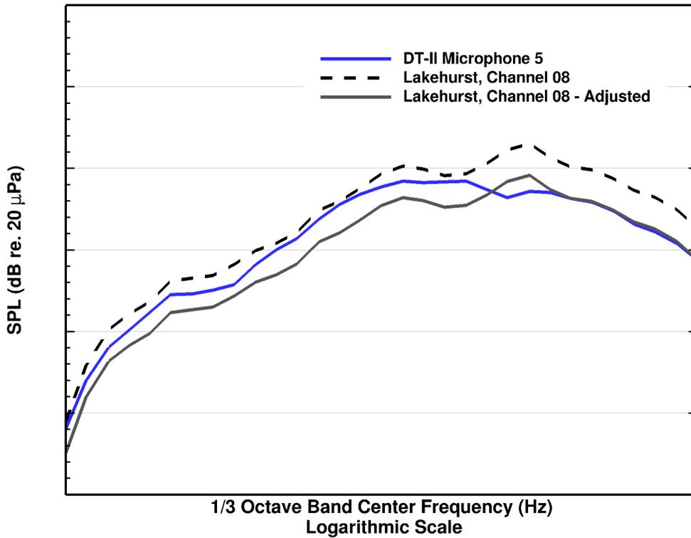
Figure 15. Comparison of land-based and carrier-based Catapult 2 military power one-third octave band spectra for the land-based microphone located at  $(x, y) = (21.0', 80.0')$ , and the carrier-based microphone at  $(x, y) = (19.1', 125.0')$ .
