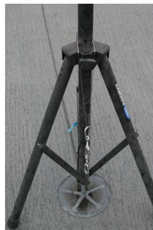
Figure 5. Microphone tripod attachment to flight deck pad-eye.
