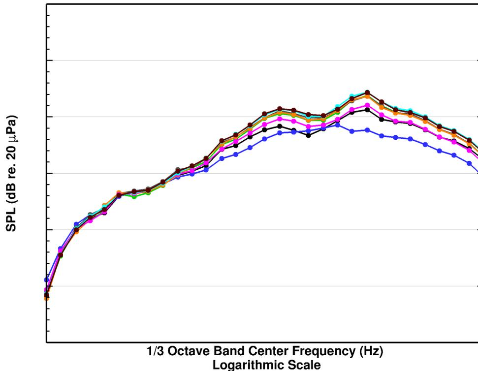
Figure 9. Catapult 2 Military power one-third octave band spectra for the microphone located at  $(x, y) = (21.0, 80.0)$ . Distances are measured in feet, and are referenced to the center of the JBD hinge line.
