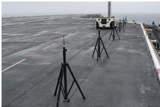
Figure 4. Microphone tripods mounted at “the Point” on the Eisenhower.
