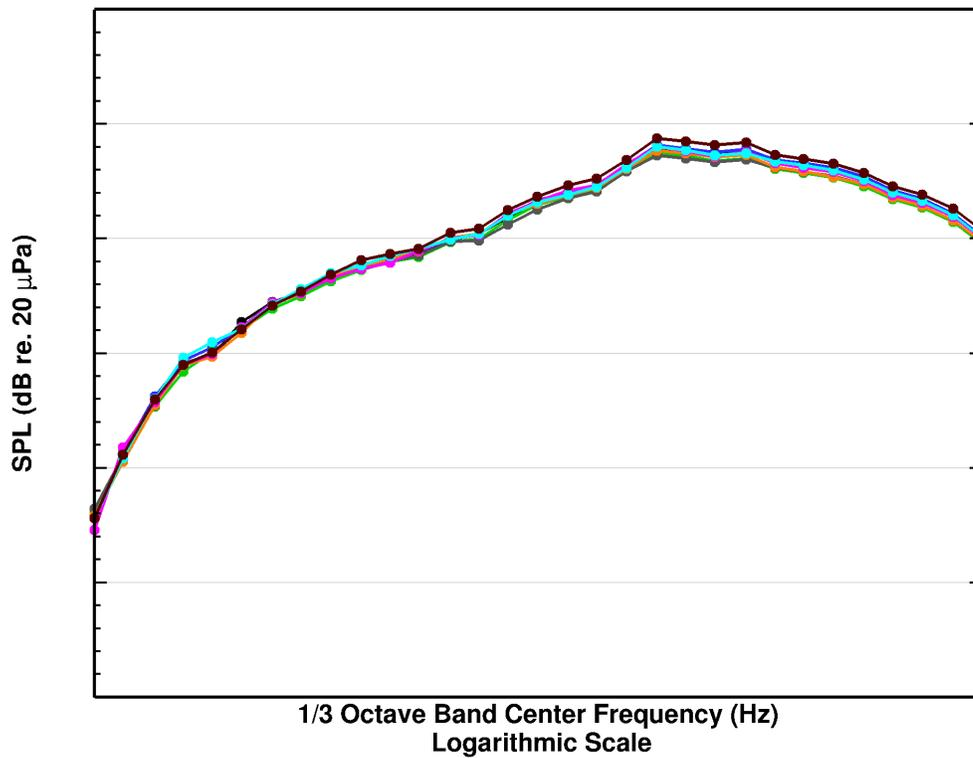
Figure 12. Land-based Catapult 1 Afterburner power one-third octave band spectra for the microphone located at  $(x, y) = (10.0, 50.0)$ . Distances are measured in feet, and are referenced to the center of the JBD hinge line.
