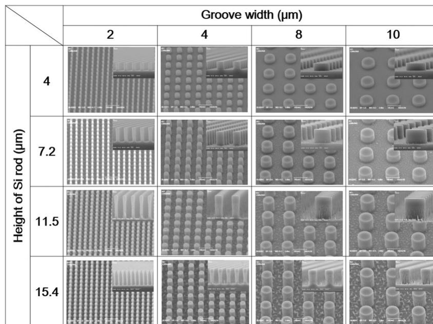
**Fig. 3.** SEM images of the Si surfaces having microscale rod structures obtained after deep Si etching. The insets show the corresponding cross-sectional SEM images. SEM was taken after the residual fluorocarbon films and  $\text{SiO}_2$  masks were removed.
