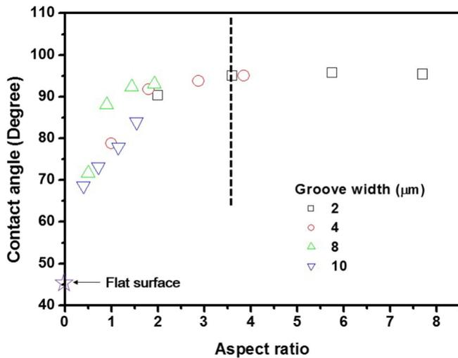
Fig. 5. Contact angles on the Si surfaces having microscale rods of various aspect ratios.
