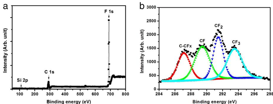
Fig. 6. (a) XPS survey scan and (b) high-resolution C 1s XPS spectra of the fluorocarbon films deposited on the microscale Si rods. The deconvolution (thin lines) of the spectra in (b) was conducted by using a linear background and Gaussian functions.
