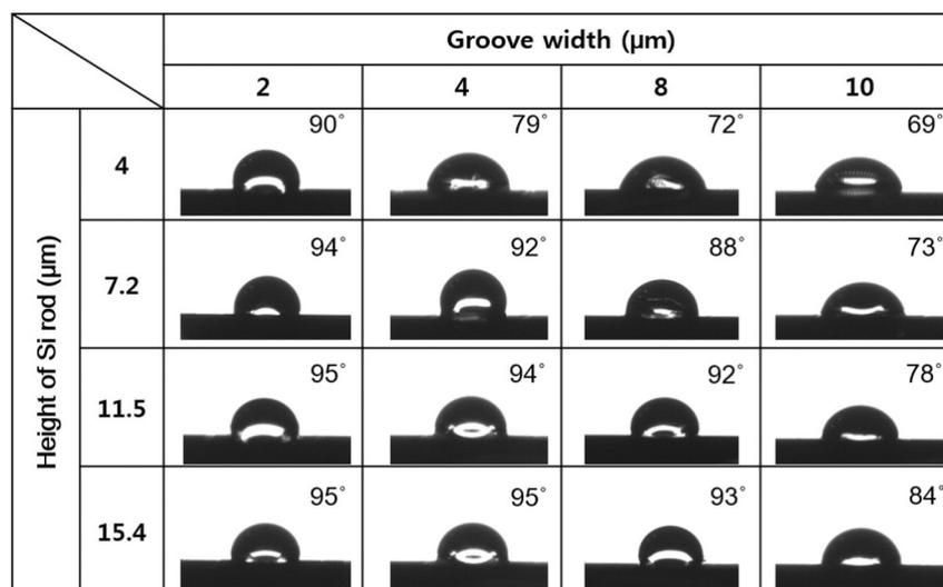
**Fig. 4.** Images of 0.5- $\mu\text{L}$  water droplets on Si surfaces having microscale rod structures. The corresponding contact angles are given in each image.
