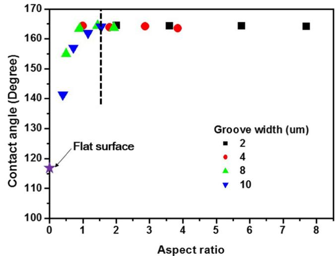
Fig. 7. Contact angles as a function of the aspect ratio of the rod, for Si surfaces having microscale rods and subsequently deposited fluorocarbon films.
