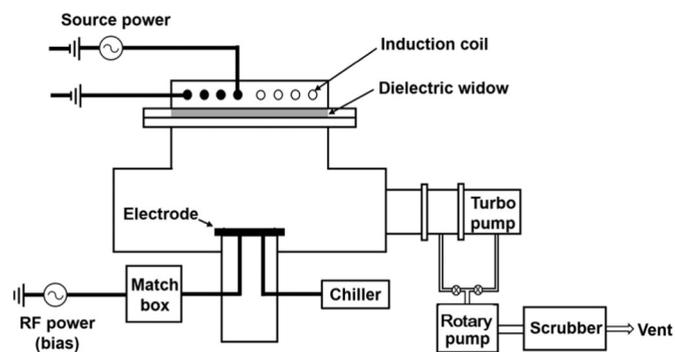
Fig. 1. A schematic of an inductively coupled plasma system used for the fabrication of microscale rod structures and the deposition of fluorocarbon films on the Si surfaces.
