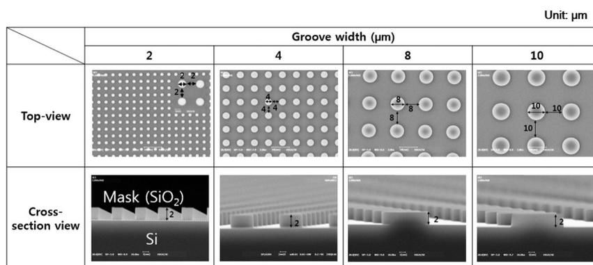
Fig. 2. SEM images of the hole patterns on the samples.  $\text{SiO}_2$  was used as a mask.
