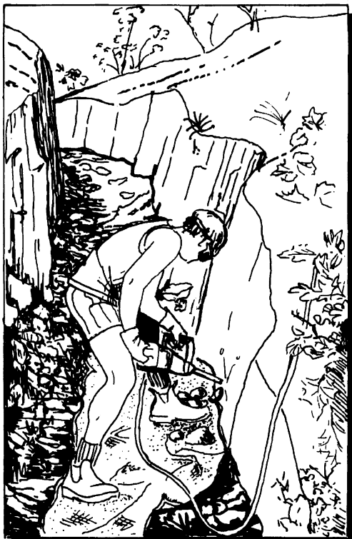
Figure 5.4 Collecting a continuous rock-chip sample from a trench wall. The sampler is using a small electric jack-hammer powered by a portable generator. The broken rock falls on to a tarpaulin laid along the floor of the trench. The same technique could be used for sampling any hard-rock exposure in the field or in a mine.
