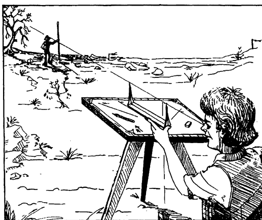
Figure 2.6 Detailed geological mapping using a plane table for survey control. In this example a simple home-made peepsight alidade is being used.
