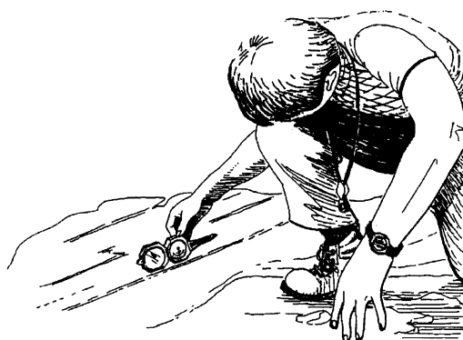
Figure C.6 Measuring the plunge of a lineation with a Brunton® compass.
