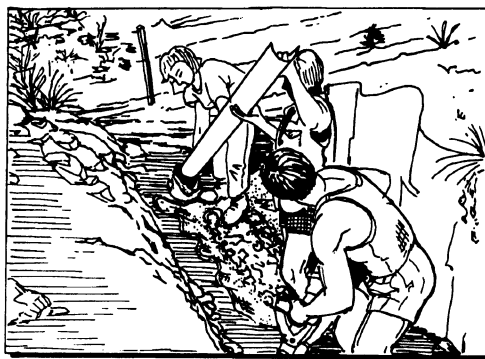
Figure 5.5 Splitting a sample for assay from an even row of small rock fragments on the ground. The rock fragments lie on a tarpaulin; a halved length of 100 mm poly-pipe is laid along the row and rocks and pipe are rolled together in the tarpaulin. Rock in the pipe is then slid into a sample bag.
