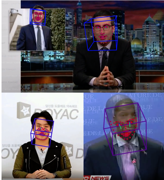
Fig. 10: Face Detection Dependency. FakeCatcher catches a fake video with multiple faces (top) as 91.7% fake, a fake video with 3% face detection confidence (left) as 99.97% fake, and a real video with 17% face detection confidence (right) as 65.47% real.
