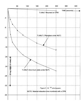
In analyzing these measurement variations, the self-dissipation of the CPM was evaluated. The CPM performance was compliant with the requirement that the CPM discharge less than 10% in 5 minutes.
