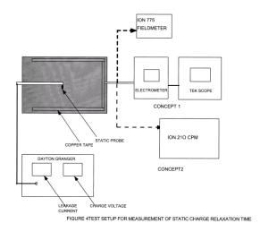
The Dayton Granger static discharger location with respect to the material was varied from 1 inch to 4 inches. The Dayton Granger charge voltage was varied from 25KV to 45KV's. From the material characterizations, one observes that these relaxation voltage curves varied by as much as 10dB for materials with the same ohms/square values. These graphs, as shown in Figures 5 through 7 are grouped, by surface resistivities, in descending order of resistivity.
