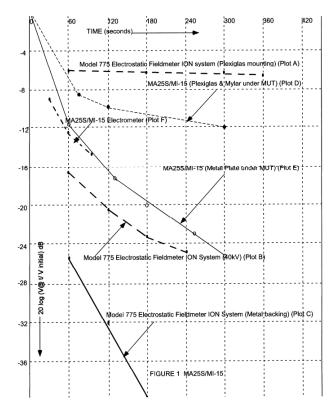
The model 775 Electrostatic Field meter placement with respect to the MA25S/MI-15 was reoriented in multiple locations in order to assess probable material uniformity. Plots A, B, and C on Figure 1 are the measurements with the ION field meter. These three plots underscore the criticality of the substructure conductivity in establishing the relaxation time of the MA25S/MI-1
