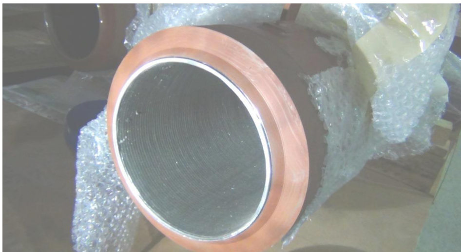
Figure 18—Spiral weld overlay in 16" pipe header
