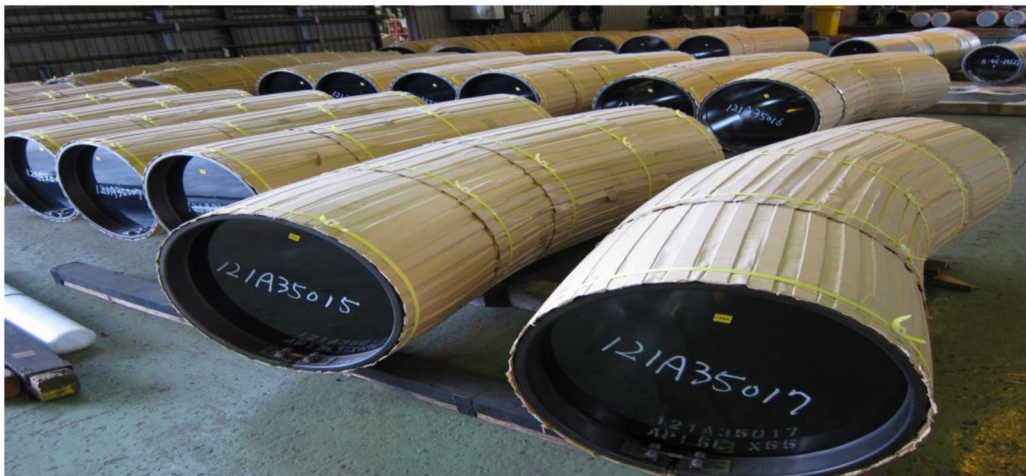
Figure 17—Induction Bends ready for dispatch
