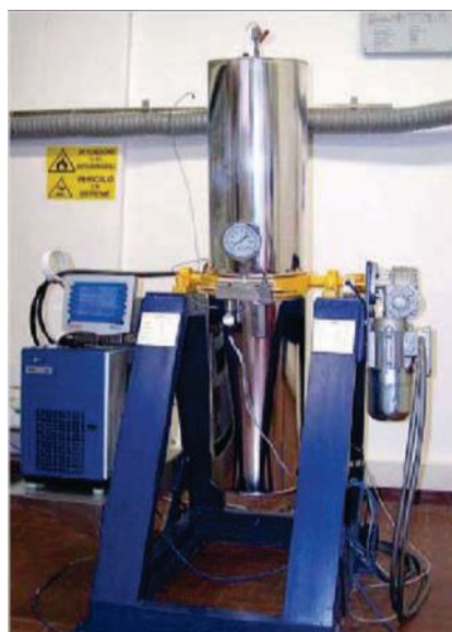
Fig. 4—An ultrahigh pressure autoclave was used to test the corrosive effects of acid gas at high and ultrahigh pressures. The materials tested were carbon steel, stainless steel, and corrosion-resistant alloys. Source: Gabetta et al. 2014.
