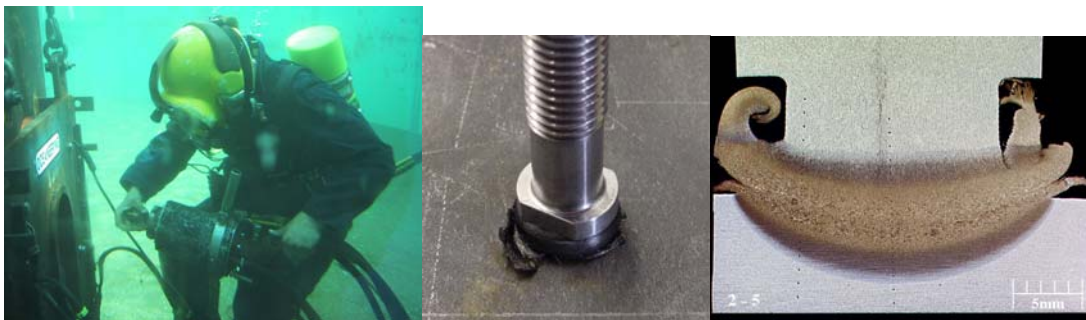
Figure 2 – Welding Equipment, Friction Stud Welded Connection and Its Micro Cross Section
