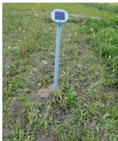
FIGURE 3. The developed sensor was installed in an open field to measure the SM.
