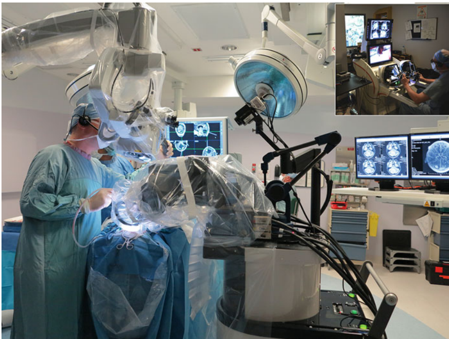
Fig. 8 The neuroArm telecapable robot developed for microsurgery (inset: the platform relocates the primary surgeon to a remote sensory-immersive workstation, here adjacent to the operating room)
