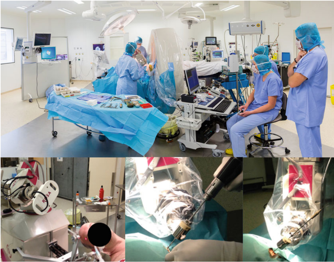
Fig. 1 Example of operating room setup (top), position of robot with respect to patient (bottom left), and use of robot to define trajectory of drilling and biopsy (bottom centre and bottom right respectively)
