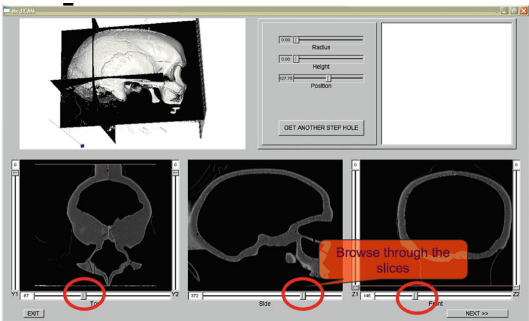
Fig. 2 Three-dimensional model of the bony anatomy is displayed in a graphic interface so the surgeon can indicate the portion of bone or soft tissue to be machined. (Reproduced with permission from Couldwell WT, MacDonald JD, Thomas CL, Hansen BC, Lapalnikar A, Thakkar B, Balaji AK (2017) Computer-aided design/computer-aided manufacturing skull base drill. Neurosurg Focus 42:E6)
