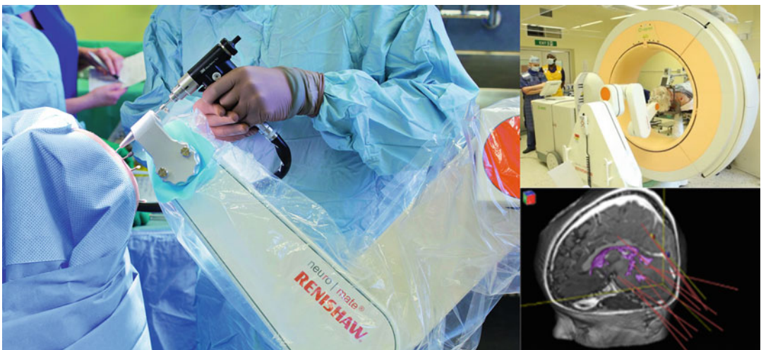
Fig. 4 The Neuromate System performing stereotactic electrode placement (inset: able to work within an imaging system for real time neurophysiologic stimulation and recording (top)); Reconstructed MR image with coordinates for target localization
