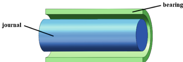
Fig. 1. Schematic of spatial revolute joint with clearance
