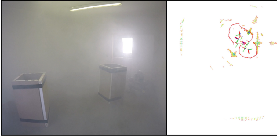
Fig. 8. Foggy environment (left) and the corresponding sensor readings (red: laser is limited by fog particles, rainbow: radar penetrates fog)
