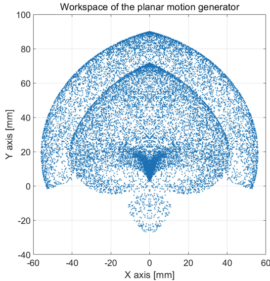
Fig. 5. The workspace of the planar motion generator
