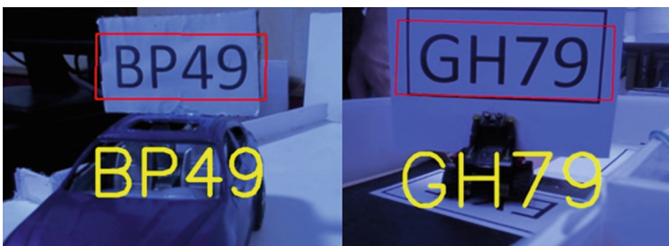
Fig. 3. Vehicle license plate number identified from an image using tesseract functions and optical character recognition.
