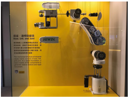
Fig. 5. Explosion display of 6-DOF industrial arm
