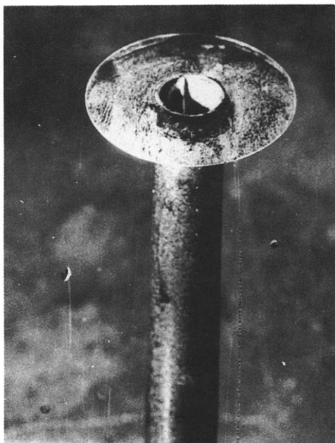
Plate 8. Flow pattern on top of a 4.0 cm wide landing platform ( d_1/d_2 = 0.328 ) at the top showing lampblack accumulation at the front and just downstream of the exit.
