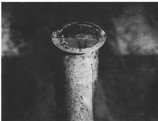
Plate 9. Flow pattern over the top of model I with exit closed and 1.0 cm wide platform ( d_1/d_2 = 0.661 ) showing reattachment of flow on the closing diaphragm.
