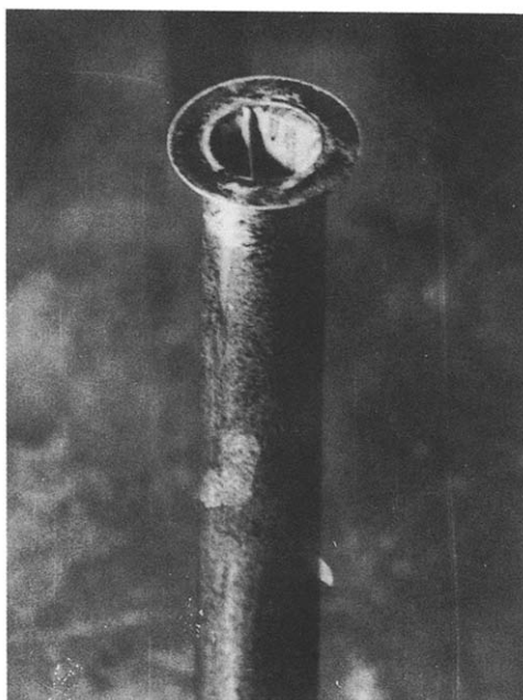
Plate 7. Flow pattern over the top of 1.0 cm wide landing platform at the top of model I showing lampblack accumulation over the whole region indicating total flow separation.
