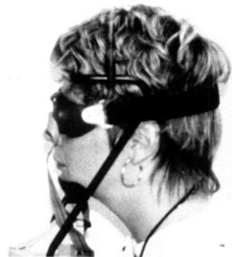
FIGURE 4: Ober2® Eye Movement Recording System utilizes goggles with microchips which track limbal eye movements by infrared reflection.
