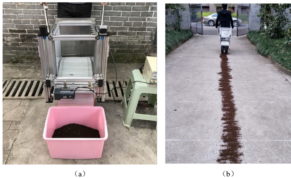
Fig. 12. Trial pictures of prototype, (a) field trial of fertilizer apparatus performance (b) field trial of overall unit.
