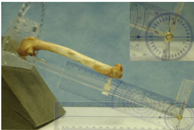
Figure 3 Positioning of the femur and custom frame with 20° distal femoral elevation. Foam wedges were used to maintain elevation and a goniometer was used to verify degree of elevation. Inset: Close up of goniometric verification of 20° elevation.
