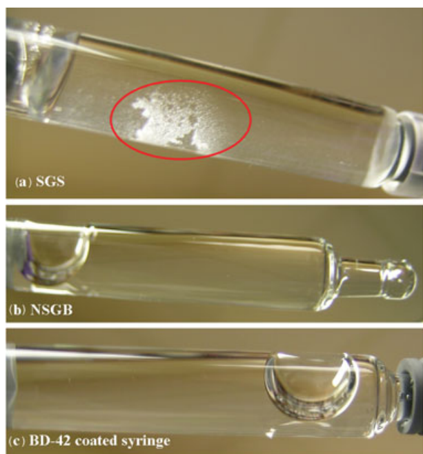
Figure 6. (a) After shaking, only SGS syringes show the development of a film on the syringe surface. (b) NSGB and (c) BD-42-coated syringes do not show any film formation.
