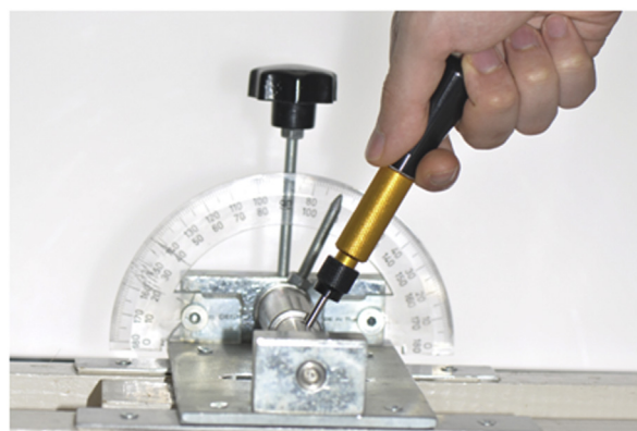
Fig 1. Insertion of an orthodontic mini-implant with the use of a screwdriver and a custom-made trestlework with goniometer to fix the bone models during insertion as well as to provide the desired insertion angle.
