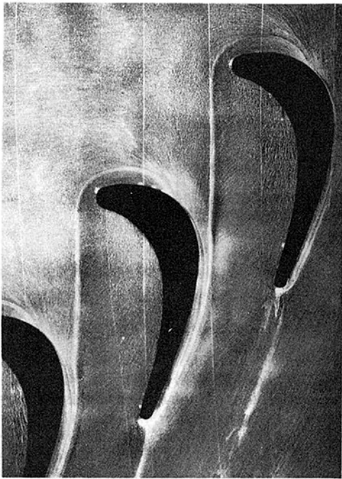
Fig. 2 Flow visualization of the limiting streamlines on the bottom wall of the cascade
