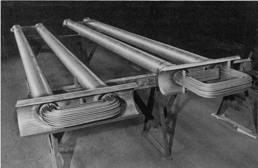
Photograph 1.e. Hairpin “regenerative” heat exchanger under fabrication. (Courtesy Joseph Oat Corporation.)
