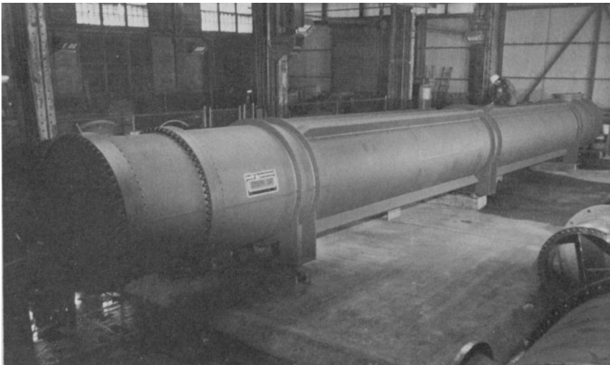
Photograph 19.b. Fixed tubesheet exchanger mounted on three horizontal saddle supports. (Courtesy Joseph Oat Corporation, Camden, N.J.)
