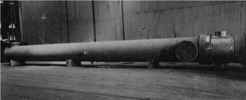
Photograph 2.a. Skirt mounted heat exchanger with a three-element joint (TEMA type BEU). (Courtesy Joseph Oat Corporation.)
